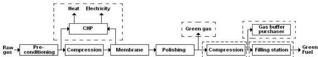
Figure 9: Schematic flow diagram of the Carborex-MS system
