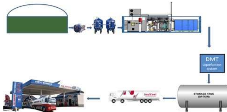
Figure 4: Configuration digester to tank station
